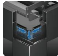
Water being flowed into post
